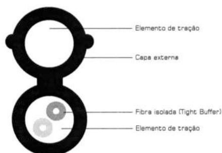
DROP TIGHT BUFFER FIG. 8 02F
